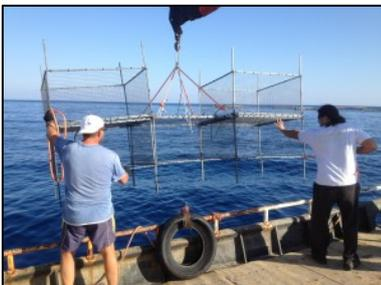
*Left: Experimental cages for IMTA operations at Seawave Fisheries.*
